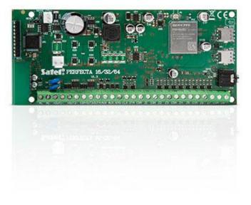
configuration of the system using the **PERFECTA Soft** program, event reporting (e.g. to a security agency monitoring station), voice telephone messaging, SMS control and audio alarm verification (listening for sounds from the protected premises). The module supports two nano–SIM cards to ensure uninterrupted communication: if transmission over the first operator's network fails, the second card is automatically selected.
